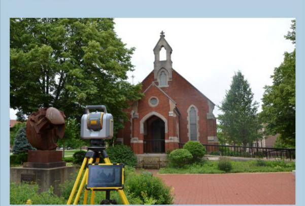
A laser scanner sends out hundreds of thousands of laser pulses per second which bounce off the buildings, lamp poles and benches and return to the sending unit. By measuring the time required for the pulse to go out and return the unit can calculate the exact location in space of the dot where the laser hit. Because the scanner sends out so many pulses, the resulting data, called a point cloud, can then be translated into a 3-dimensional model of the surroundings.
